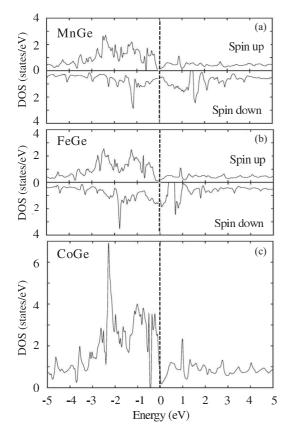
FIG. 16. DOS for MnGe, FeGe, and CoGe: Density of states (DOS) for both the majority (spin-up) and minority (spin-down) subbands of MnGe and FeGe, as well as the DOS of CoGe calculated at the experimental lattice constants.
