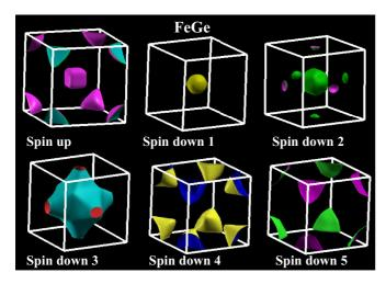
FIG. 21. (Color online) Fermi surface of FeGe: The majority-spin subbands (spin up) are shown in the top left frame and the five minority-spin subbands (spin down) are displayed in remaining frames.
