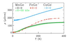
FIG. 12. (Color online) Resistivity: Resistivity  $\rho$  vs temperature T at fields H identified in the figure for FeGe, MnGe, and CoGe.
