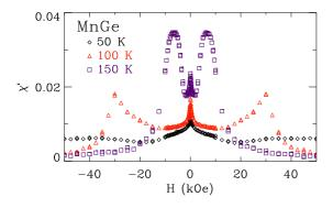
FIG. 7. (Color online) Field dependence of the ac susceptibility: The real part of the ac susceptibility  $\chi'$  of MnGe at three temperatures demonstrating the rich structure and sharp transitions that occur with field H below the Curie temperature.
