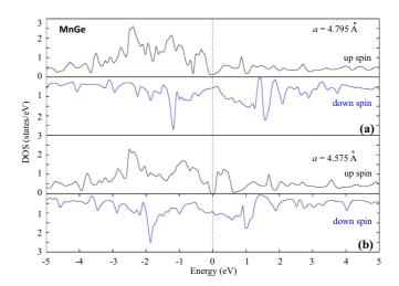
FIG. 15. (Color online) DOS for MnGe for two different lattice spacings: Density of states (DOS) for both the majority (spin-up) and minority (spin-down) subbands calculated at the experimental lattice constant (a) and at a smaller lattice constant (b).
