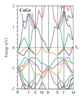
FIG. 19. (Color) Band structure of CoGe: Energy bands calculated at points of high symmetry.
