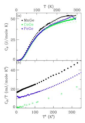
FIG. 10. (Color online) Specific heat: (a) Specific heat  $C_P$  vs temperature T of MnGe, FeGe, and CoGe at zero field. Dashed lines are fits of a model for the phonon contribution to C(T) that includes Debye and Einstein terms. (b)  $C_P/T$  vs  $T^2$  at zero field and low temperatures.
