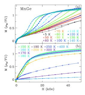
FIG. 5. (Color online) Magnetization: Magnetic field H dependence of the magnetization M for MnGe at temperatures between 5 and 140 K (a) and between 150 and 400 K (b) as indicated in the figure. Lines connect the data points for display purposes. The hysteresis at low temperatures is apparent in the data at 5 K where both the initial increasing H magnetization (lower data) and the subsequent decreasing H sweep (upper data) are shown.
