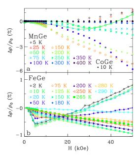
FIG. 13. (Color online) Magnetoresistance: (a) Magnetoresistance  $\Delta \rho/\rho_0 = [\rho(H) - \rho_0]/\rho_0$ , where  $\rho_0$  is the zero-field resistivity, of MnGe and CoGe at temperatures indicated in the figure. The hysteresis at low temperatures is demonstrated by the 50-K data where both the increasing and decreasing field data are shown. (b)  $\Delta \rho/\rho_0$  for FeGe at temperatures indicated in the figure. Lines connect the data points for display purposes.
