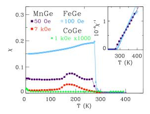
FIG. 3. (Color online) Magnetic susceptibility: dc magnetic susceptibility  $\chi$  vs temperature T for FeGe, MnGe, and CoGe at magnetic fields indicated in the figure. Note that the CoGe data have been multiplied by a factor of 1000 for clarity. Inset:  $\chi^{-1}$  vs T for FeGe and MnGe. Lines represent fits to Curie-Weiss behavior and correspond to Weiss temperatures of 284 and 270 K and magnetic moments of 1.0 and 1.35  $\mu_B$  per formula unit for FeGe and MnGe, respectively.
