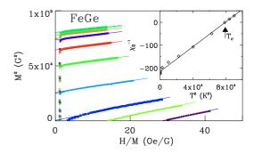
FIG. 8. (Color online) Arrott plot for FeGe: The square of the magnetization  $M^2$  plotted vs the ratio of the magnetic field H to M to compare with a standard mean-field form of M commonly known as an Arrott plot [40]. Symbols are the same as in Fig. 6. Solid lines are linear fits to the high-field behavior. Inset: plot of the H/M intercepts  $\chi_0^{-1}$  of linear fits in the main frame to determine the Curie temperature  $T_c$  as indicated in the figure.
