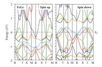
FIG. 18. (Color) Band structure of majority (spin-up) and minority (spin-down) spin subbands of FeGe: Energy bands calculated at points of high symmetry at the experimental lattice constant.
