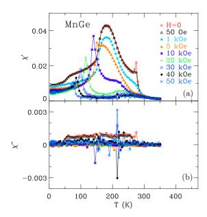
FIG. 4. (Color online) ac magnetic susceptibility: (a) Real  $\chi'$  and (b) imaginary  $\chi''$  parts of the ac magnetic susceptibility vs T for MnGe at magnetic fields indicated in the figure. Lines connect the data points for display purposes.
