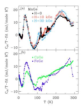
FIG. 11. (Color online) Specific heat after subtraction of a model for the phonon contributions: (a)  $C_P/T$  of MnGe at fields identified in the figure after subtraction of the model represented by the dashed line in Fig. 10(a) vs T. Several phase transitions are apparent. (b)  $C_P/T$  vs  $T^2$  for FeGe and CoGe at zero field after subtraction of the model represented by the dashed lines in Fig. 10(a). Lines connect the data points for display purposes.
