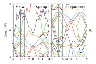
FIG. 17. (Color) Band structure of the majority (spin-up) and minority (spin-down) subbands of MnGe: Energy bands calculated at points of high symmetry at the equilibrium lattice constant.
